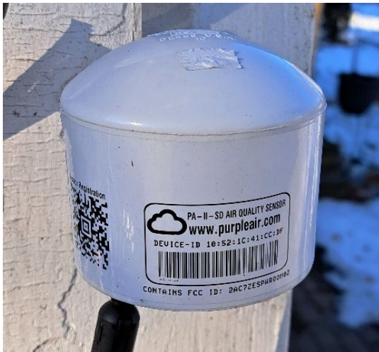
Figure 10: PurpleAir PA-II Monitor
